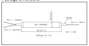
The optical path of forward pump type for pass wavelength is from port 3 to port 1, same direction as reflect wavelength (pump light).
